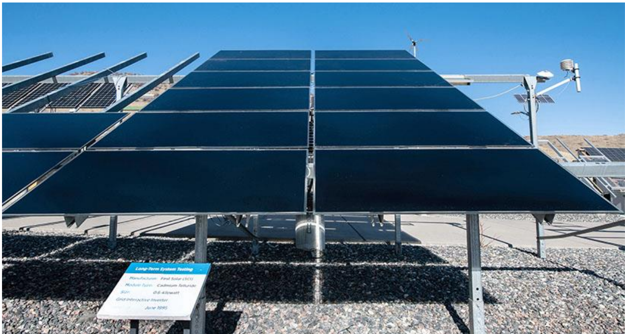
A 0.6-kW First Solar cadmium telluride photovoltaic test array was installed in June 1995 at NREL's Outdoor Test Facility. Photo by Dennis Schroeder, NREL
